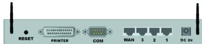
Figure 2-2 Rear Panel Ports
