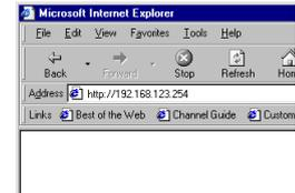
2. In the "Location" field (for Netscape) or "Address" field (for Internet Explorer), type "http://192.168.123.254" and press <ENTER>.
